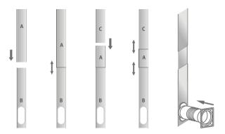
**Step 4:** Close your window to secure the kit in place. It needs to hold the windows kit firmly in place, secure the window kit with duct tape if required. It is recommended that the gap between the adapter and the sides of the window should be sealed off for maximum efficiency.
