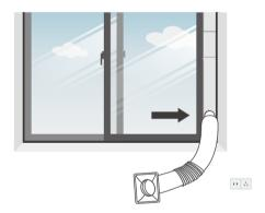
**Step 5:** Attach the hose connector to the exhaust air outlet of unit.
