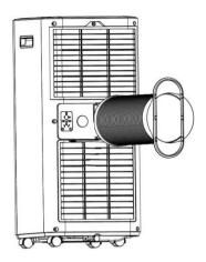
**Step 6:** Adjust the length of the flexible exhaust , to make sure the distance between the unit and the window will be more than 70cm, and the height from the exhaust hose to the floor will be more than 90cm. And avoid bends in the hose. Then place AC near an electrical outlet.
