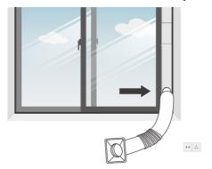
Step 5: Attach the hose connector to the exhaust air outlet of unit.
