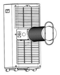
**Step 6:** Adjust the length of the flexible exhaust hose to make sure the distance between the unit and the window will be more than 70cm, and the height from the exhaust hose to the floor will be more than 90cm. And avoid bends in the hose. Then place AC near an electrical outlet.
