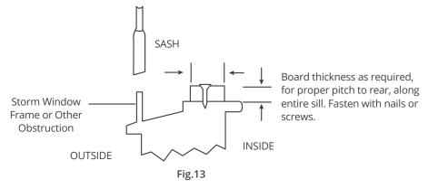
If Storm Window Frame must remain, be sure the drain holes or slots are not caulked or painted shut. Accumulated Rain Water or Condensation must be allowed to drain out.
