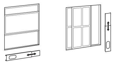
Adjust the length of the window slider kit according to your window, and then secure the position with the provided screws.
