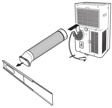
Slide the hose connector to the air exhaust on the unit, and attach the window kit adapter to the window slider kit
