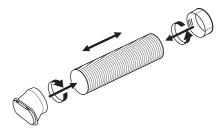
· Connect the exhaust hose to the hose connector and window kit adapter.
