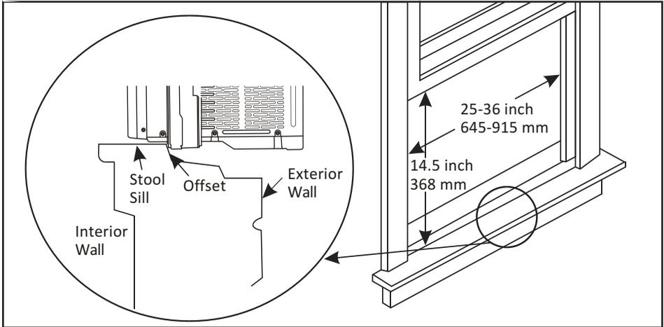
1. This air conditioner is designed to be installed in a standard single-hung or double-hung window with a window width between 25" and 36" (645mm - 915mm).
